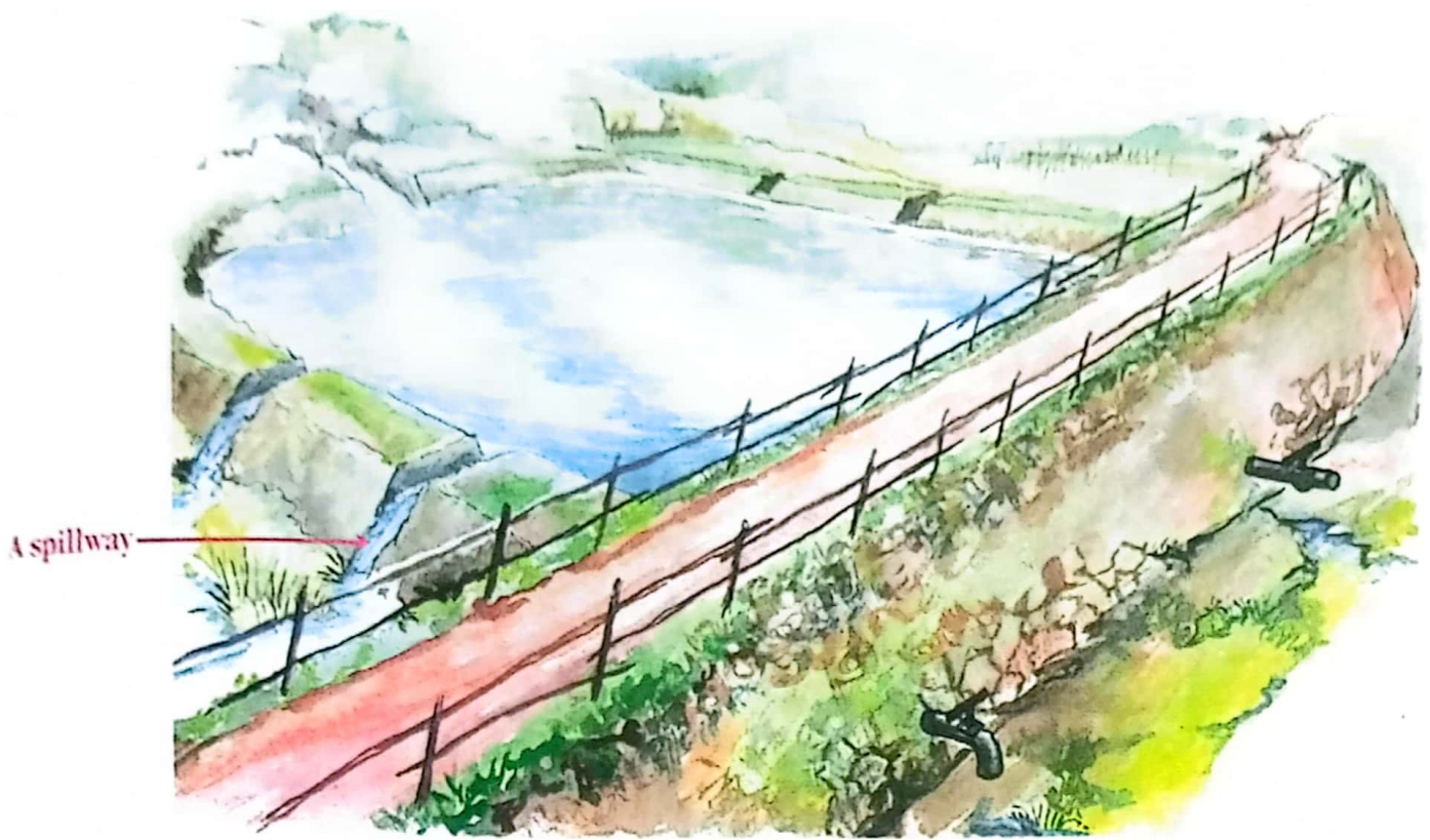
A valley dam with a concrete spillway.
